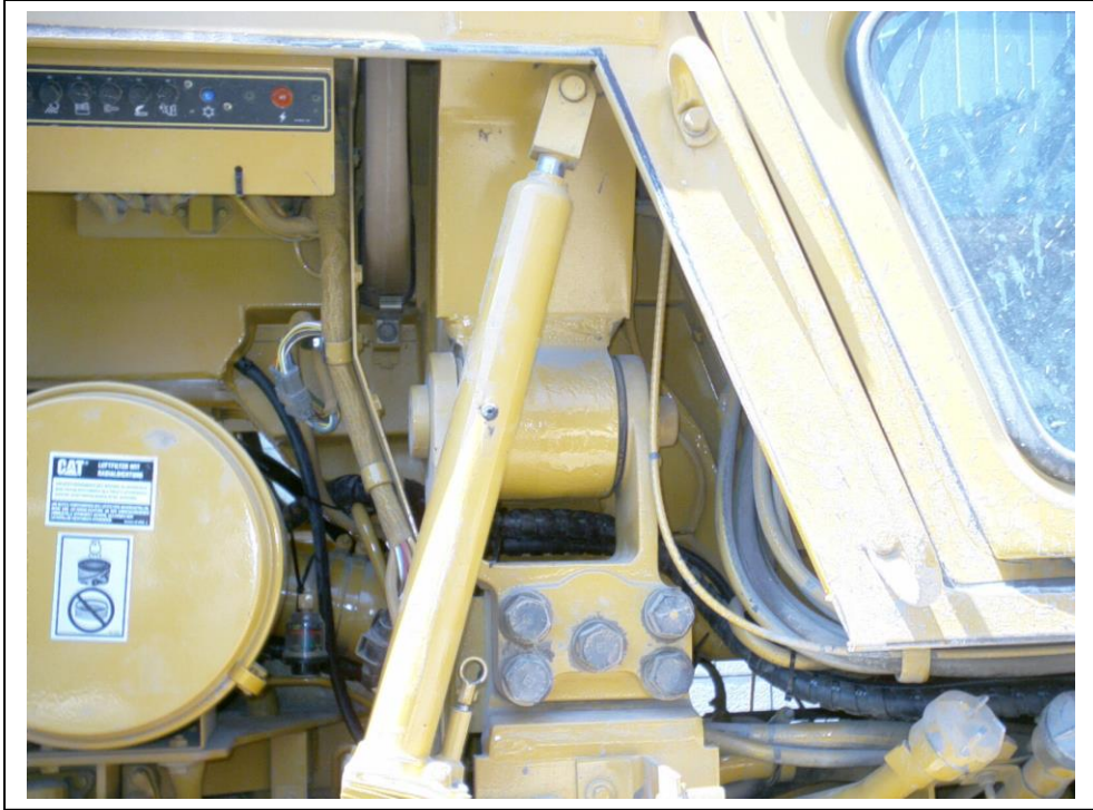
Hose routing to opening in bottom of cab. Run so that the cab can be tilted up.
